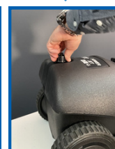
Chemical / Detergent Inlet
