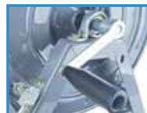
DIRECT HAND CRANK REWIND WITH LOCKING PIN
