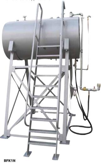
Bottom fill kit includes: Fittings, valves, camlocks, 2 x 900mm 1½" gal pipe pieces, 200mm pipe piece, tee, 2 pipe brackets with all thread, 2" plug for adding fuel additives if required and thread tap. Designed for easy installation to standard tripod or horizontal style tanks where fill point is within 200mm from tank edge and overall height maximum is 3.2mt.
